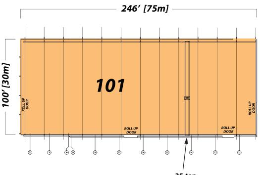
Specifications Length: 246' Width: 100' Eave Height: 36' Clear Height: 35' Crane Hook Height: 22' Floor Depth: Varies 8"-12" 1 Drive-in Door Offices are Build-to-Suit: 3,000 SF of office space is available but not included Crane Service: 25-Ton 25-ton overhead crane
